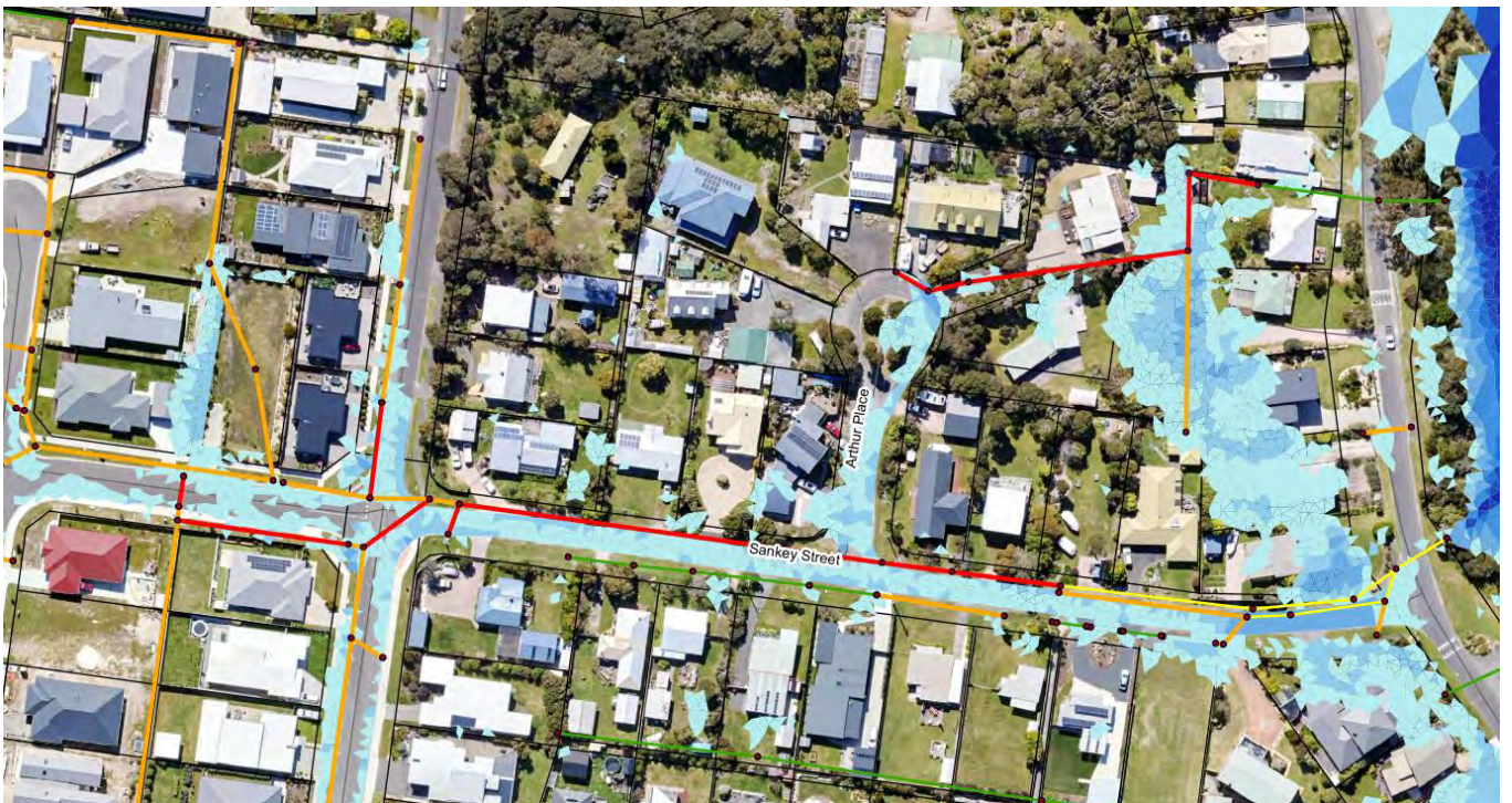
Figure 14 Major storm (1% AEP) event – Option 1 retain/upsized detention basin – extract of flood map from Appendix A
