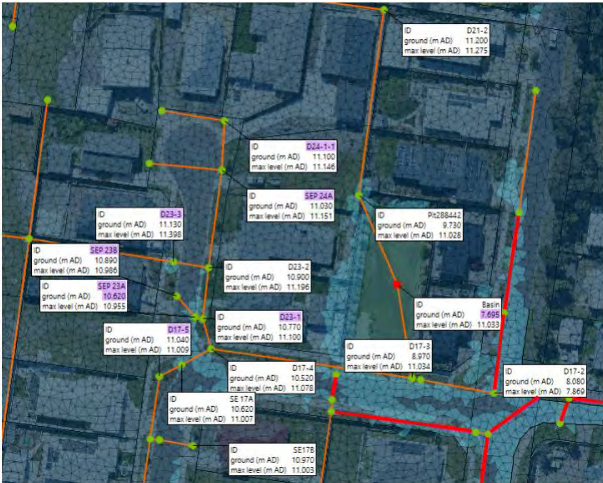
Figure 20 Major storm (1% AEP) event with CCF - option 1 retain/upsized detention basin - ground levels and maximum water levels
