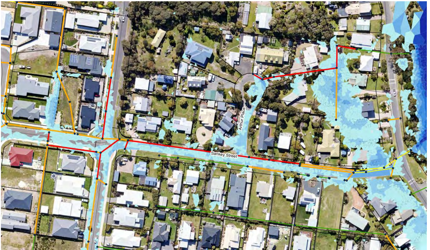
Figure 21 Figure 22 major storm (1% AEP) event with CCF - option 1 retain/upsized detention basin - extract of flood map from Appendix A
