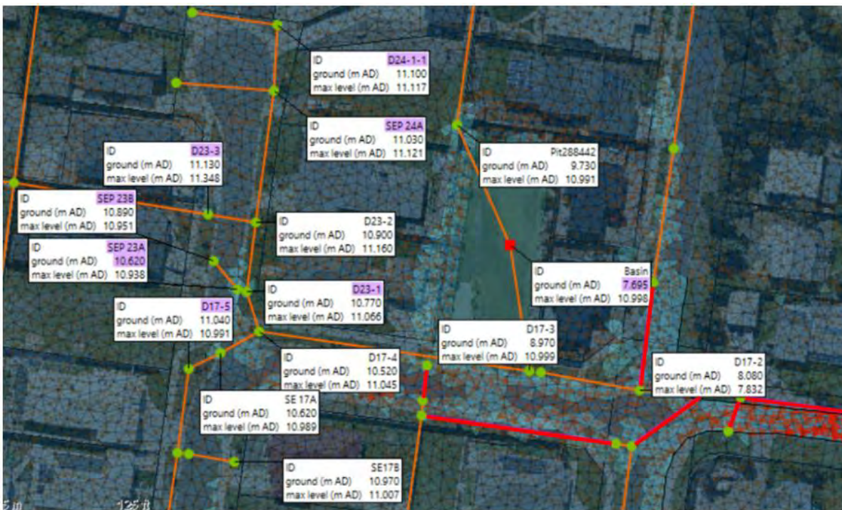
Figure 16 Major storm (1% AEP) event – option 1 retain/upsized detention basin – ground levels and maximum water levels
