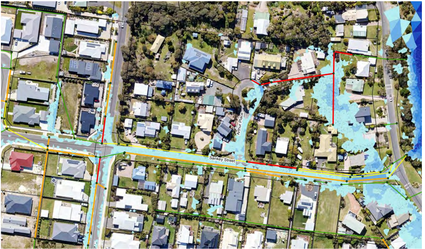
Figure 23 Major storm (1% AEP) event with CCF – option 2 removing detention basin - extract of flood map from Appendix A
