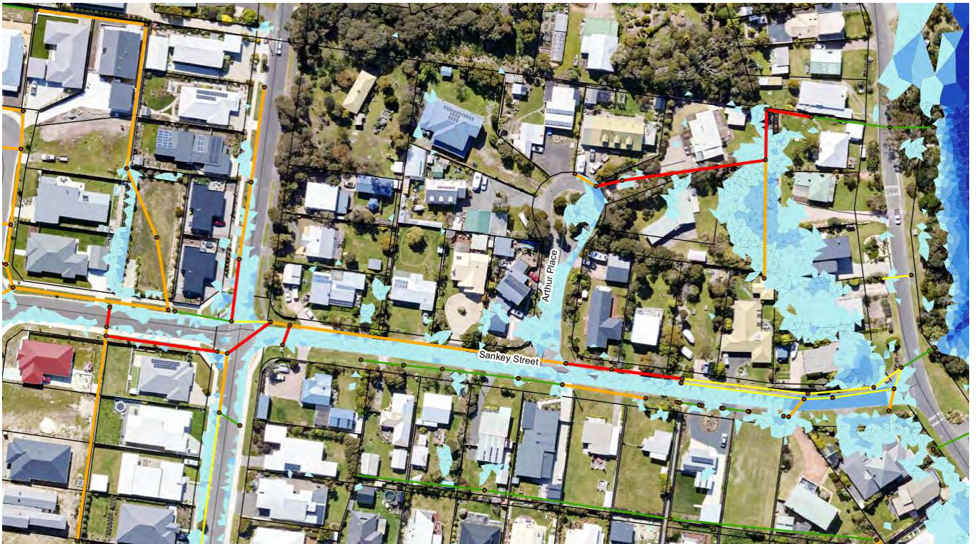
Figure 13 Minor storm (10% AEP) event – Option 1 retain/upsized detention basin - extract of flood map from Appendix A
