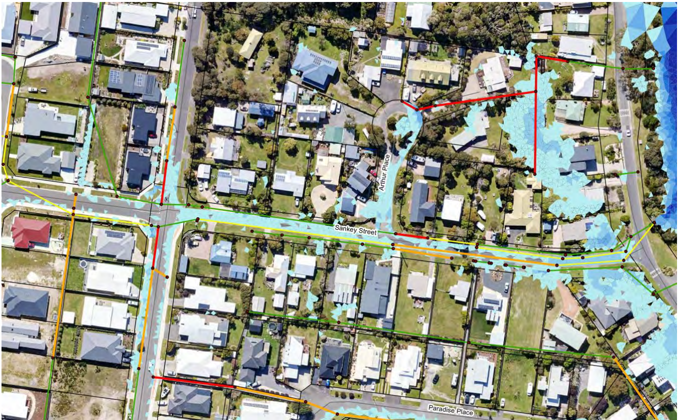
Figure 19 Major storm (1% AEP) event – option 2 removing detention basin - extract of flood map from Appendix A
